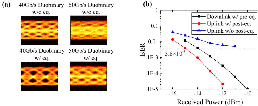
Fig. 10. (a) Uplink duobinary eye diagrams w/ and w/o post-equalization when data rate is  $40\text{Gb/s}$  and  $50\text{Gb/s}$ , (b) downlink and uplink BER performances of  $40\text{Gb/s}$  duobinary signals
