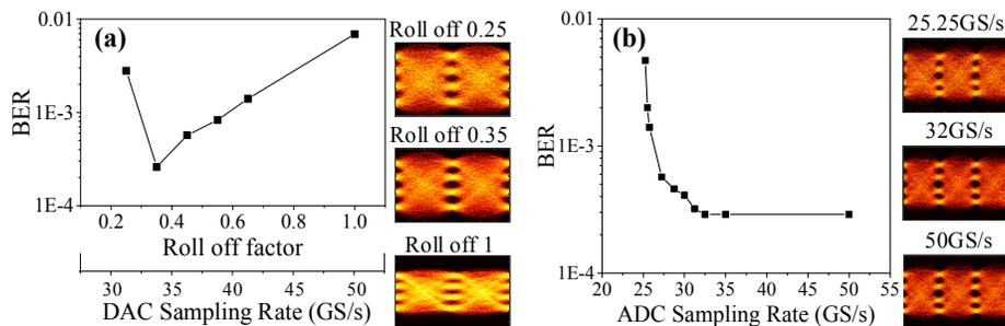
Fig. 6. (a) Impact of the downlink roll off factor on the BER performance and the corresponding required DAC sampling rate, (b) BER performance versus uplink ADC sampling rate.
