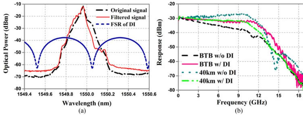
Fig. 4. (a) The optical spectra of one downstream wavelength with and without DI and (b) downstream frequency response with and without DI.
