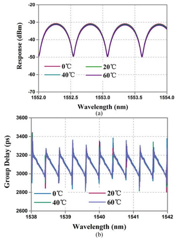
Fig. 3. (a) Spectral response of DI under different temperatures and (b) Group delay profile of FBG under different temperatures.
