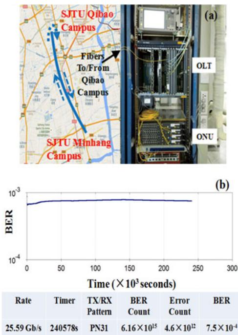
Fig. 10. (a) Map of the round-trip link in SJTU and photo of the 100-Gb/s TWDM-PON systems; (b) BER performance of the downstream signal during 67-h real-time measurement.
