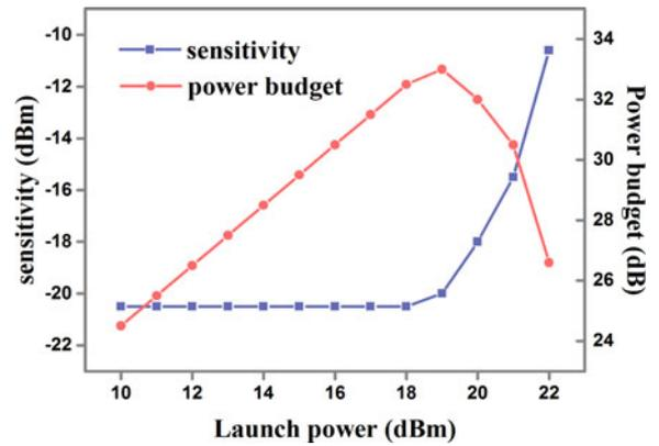
Fig. 8. Required optical power over 40 km SMF for a BER of  $10^{-3}$  versus launch power.
