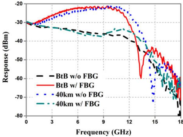
Fig. 5. Upstream frequency response with and without FBG.
